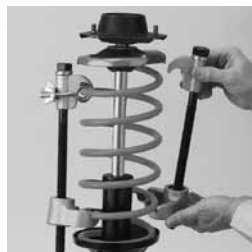
1. Attach clamps to spring
