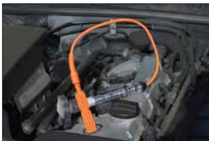
Test coil directly to ground
