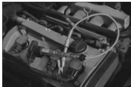
Test coil directly to ground
